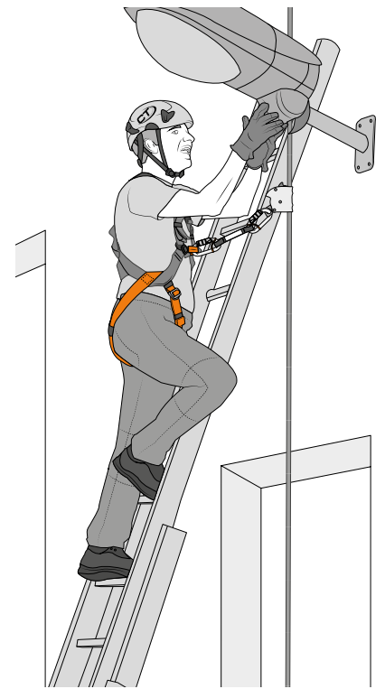
9.3 - Working on a ladder
