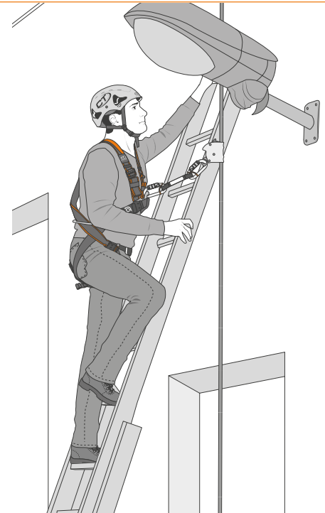
11.3 - Working on a ladder
