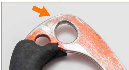
Worn body next to the lower attachment hole.
