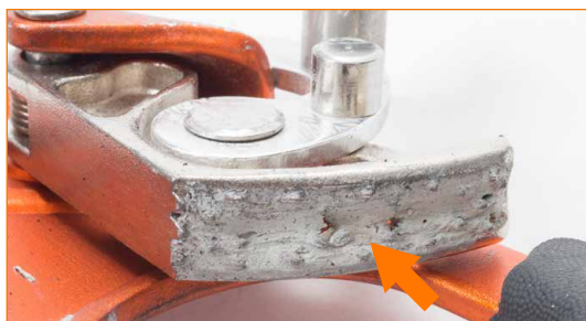
Locking cam with missing and broken teeth due to a strong wear and to improper uses.
