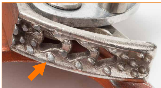
Locking cam with missing and broken teeth due to a strong wear and to improper uses.
