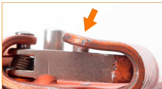
Deformed body due to the accumulation of rope sheathes after a fall with F_f > 1 .
