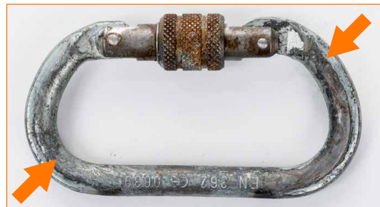
Connector with clear incision/cut on body.
