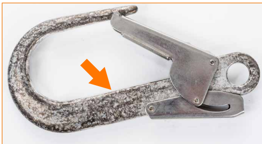
Double-lever connector with clear signs of corrosion.
