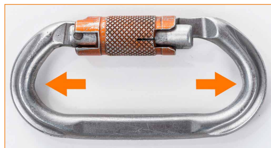
Connector with screw-up locking sleeve extremely deformed due to incorrect use.
