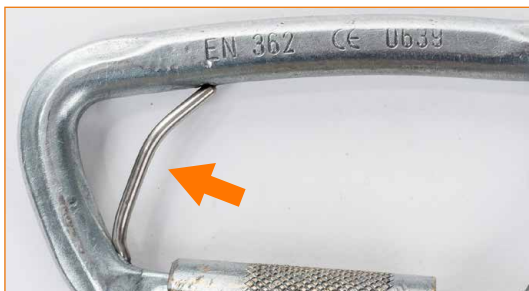
Connector with deformed ACL bar.
