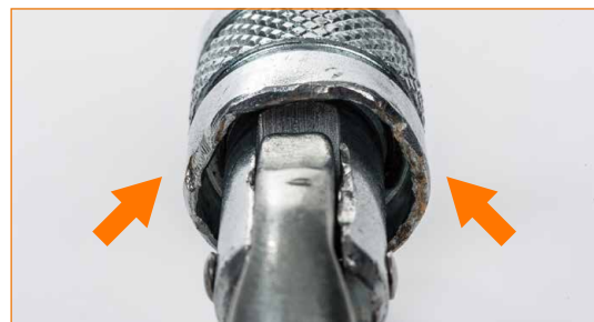
Connector with heavily damaged screw gate.
