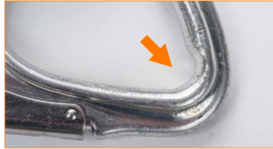
Body with distinct signs of use in area subject to wear.
