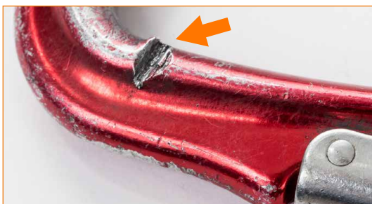
Connector with screw-up locking sleeve showing clear signs of oxidation.
